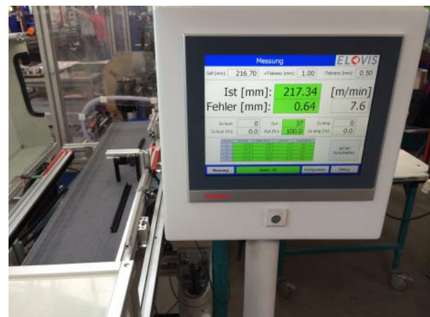
Fig. 20: SLM-SPS sorting control
