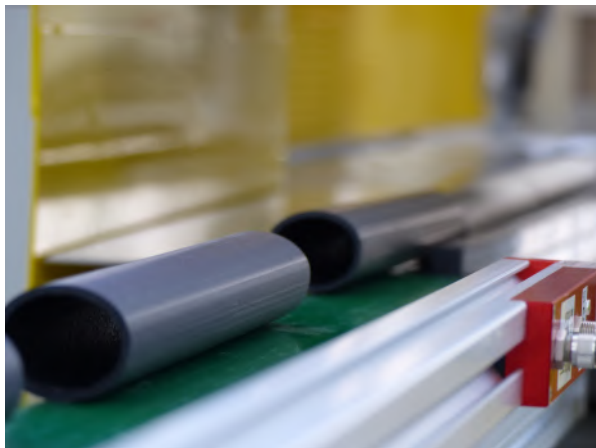
Fig. 6: Measurement of extruded tubes
